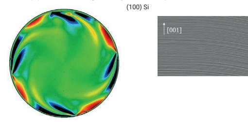
Wafer showing a ring-like global stress field superimposed by eddies arising from the melt-crucible rotation. High-resolved shear stress map showing growth striations which represent a concave phase boundary on a slice cut in growth direction. Native birefringence and global fields have been eliminated by high-pass filtering.
